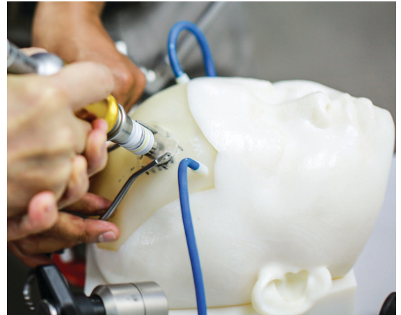
Figure 8 - This multi-material model allows physicians to train on neurosurgery procedures using the same devices and techniques used in live patient cases. Courtesy of the Centre for Biomedical Technology and Integration.
