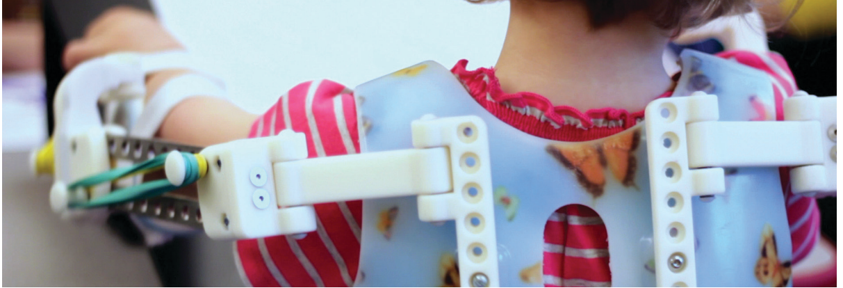
Figure 12 - Emma's smaller, customized WREX, developed using FDM technology.
