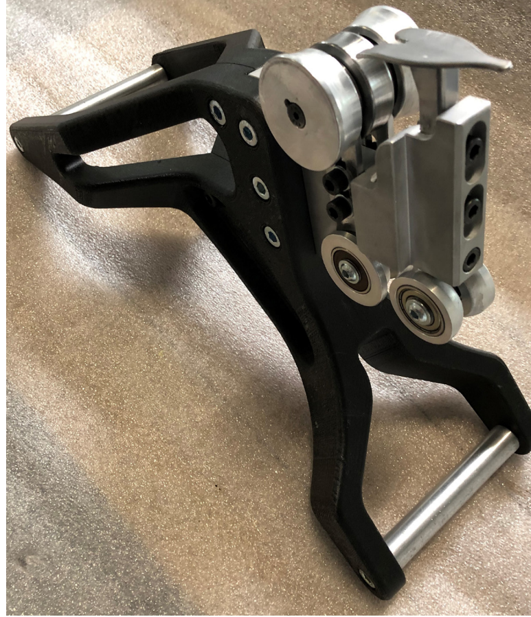
RUSTIN used FDM Nylon 12CF material to create this device for mounting windshield seals in trams for the Frankfurt Transport Company.
