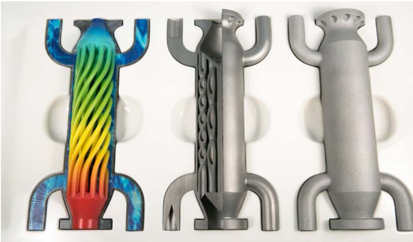
Proof-of-concept models 3D printed in color plastic and metals help validate designs quickly.
