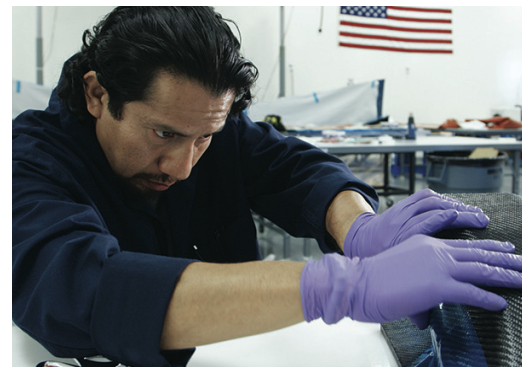
Prior to bagging for cure, the ply lay-up is completed.
