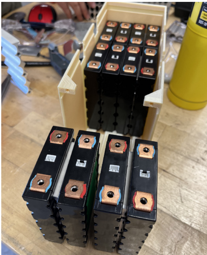
The accumulator module, with sections printed using ULTEM™ 1010 resin.
