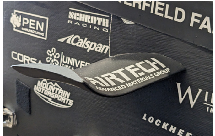
One of the car's 3D printed aerodynamic whiskers.
