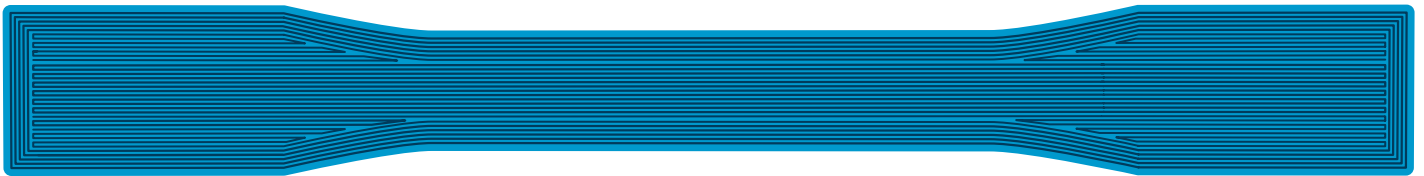
Figure 6- Toolpaths of D638 tensile coupon with unidirectional toolpaths within the necked region.
